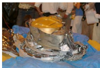
Figure 1: The condition of the science canister after it was retrieved from the field and brought to the high-bay at UTTR.
